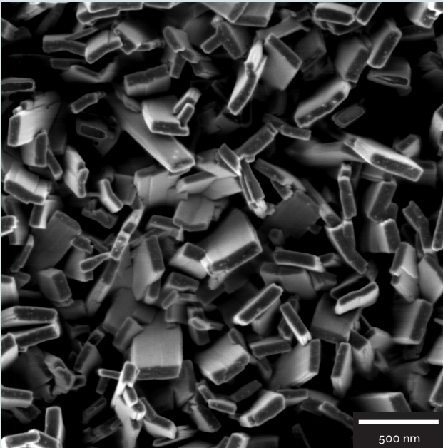
Fig. 3, 4: Sodium oxide-nitrite crystals synthesized by hydrothermal treatment of titanium substrate in sodium hydroxide solution under nitrogen.
