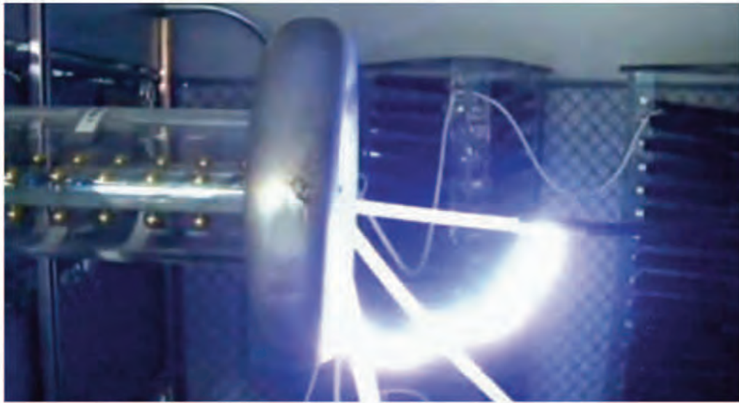
Figure 9. CUT#4. Photo of flashover. Positive polarity.
