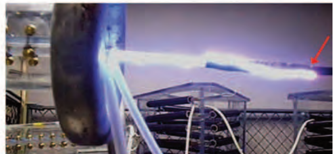
Figure 11. CUT#6. Photo of flashover. Positive polarity.
