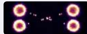
Quadruple trap configuration, allowing for complex DNA-DNA experiments.
