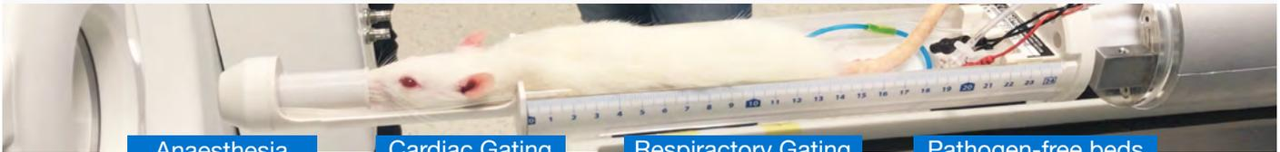
The Imaging beds on MR SOLUTIONS systems are designed to provide important support functions to the animal during the preparation stage and throughout the imaging process. The beds provide anaesthetic gas to the animal and thermo-regulation of the animal during the scan.
